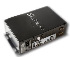
The Vision Lane Computer (VLC) is the heart of our scoring system utilizing the highest quality components. Each pair of lanes consists of one VLC, one API, one Pin Cam, and one or two QWERTY keypads, or High definition touch screens. This system is networked to our Focus-NEX Front Desk and back office system.
